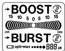
Power Bar: This shows the output from 0 to 15 for both left and right channels. Each segment represents approximately 7% of the total output.
