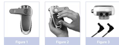
Inserting the battery Press and rotate the belt clip to reveal the battery compartment.
